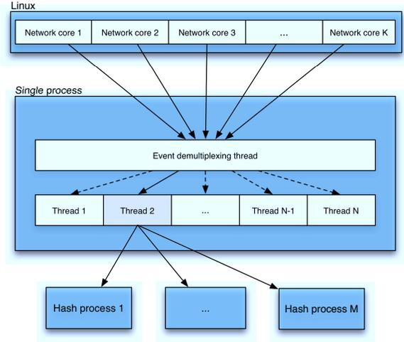
Figure 5: Execution model of Memcached on TILEPro64.
