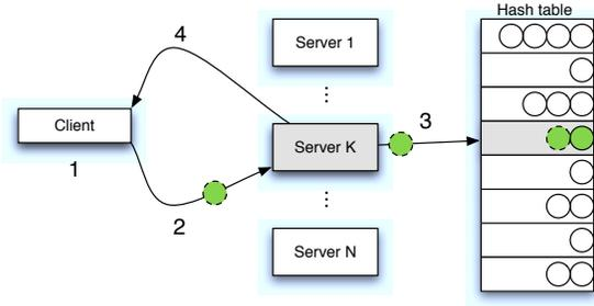
Figure 1: Write path: The client selects a server (1) by computing  $k_1 = \text{consistent\_hash}_1(\text{key})$  and sends (2) it the (*key, value*) pair. The server then calculates  $k_2 = \text{hash}_2(\text{key}) \bmod M$  using a different hash function and stores (3) the entire (*key, value*) pair in the appropriate slot  $k_2$  in the hash table, using chaining in case of conflicts. Finally, the server acknowledges (4) the operation to the client.
