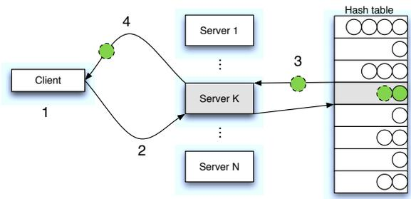
Figure 2: Read path: The client selects a server (1) by computing  $k_1 = \text{consistent\_hash}_1(\text{key})$  and sends (2) it the *key*. The server calculates  $k_2 = \text{hash}_2(\text{key}) \bmod M$  and looks up (3) a (*key, value*) pair in the appropriate slot  $k_2$  in the hash table (and walks the chain of items if there were any collisions). Finally, the server returns (4) the (*key, value*) to the client or notifies it of the missing record.
