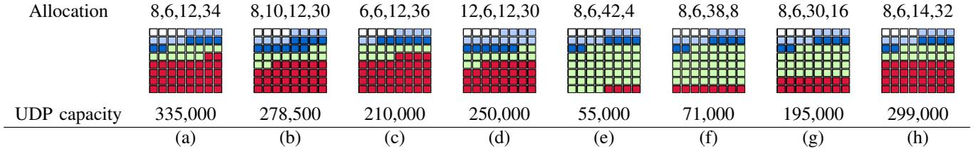
Figure 7: Read capacity at various core allocations. the numbers in each sequence represent the cores allocated to network workers (light blue), hash table (dark blue), TCP (green), and UDP (red), respectively. Linux always runs on 4 cores (white).
