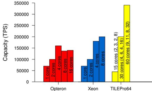
Figure 8: Scalability of different architectures under increasing number of cores. For x86, we simply change the number of Memcached threads with the `-t` parameter, since threads are pinned to individual cores. For TILEPro64, we turn off a number of cores and reallocate threads as in Fig. 7.
