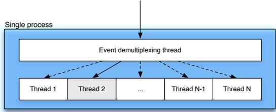
Figure 4: Execution model of standard version of Memcached.
